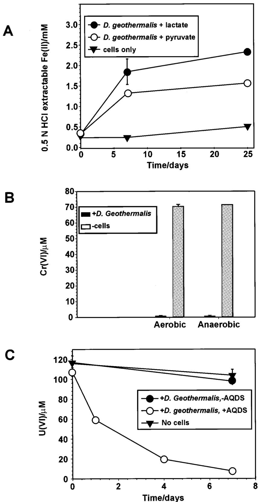
FIG. 3. Metalloredox by wild-type *D. geothermalis*. (A) Fe(III)-NTA reduction coupled to oxidation of organic substrates at 45°C in the absence of oxygen. (B) Cr(VI) reduction in aerobic or anaerobic conditions as measured by loss of Cr(VI) from solution at 40°C. (C) Reduction of U(VI) in the presence or absence of AQDS as measured by loss of U(VI) at 40°C.
